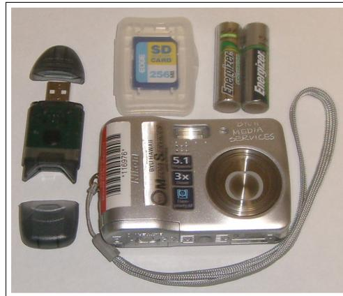
On the top center of this picture, we see an SD card. This is the kind that I make available to you. It has limited capacity, 256 MB, and will hold about 200 pictures at maximum resolution, depending on lighting.
